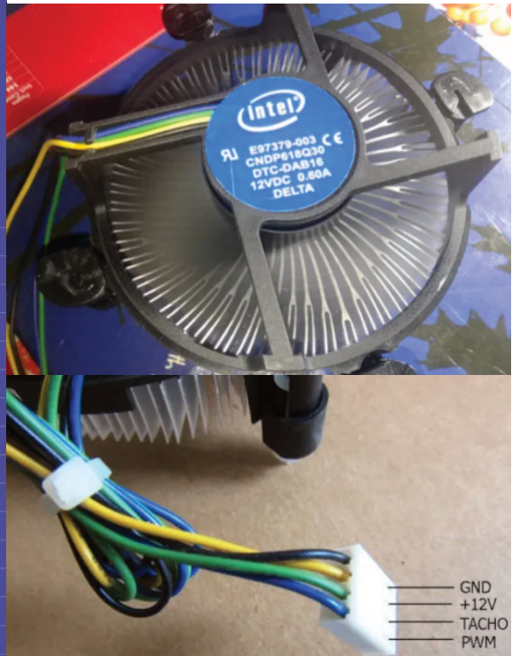
Slika 4.3. CPU ventilator pinout
